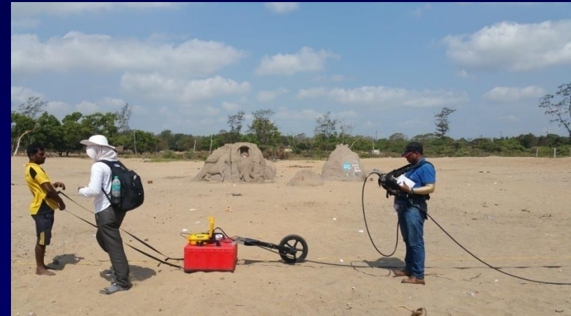
GPR survey to locate structures buried in south of the temple
